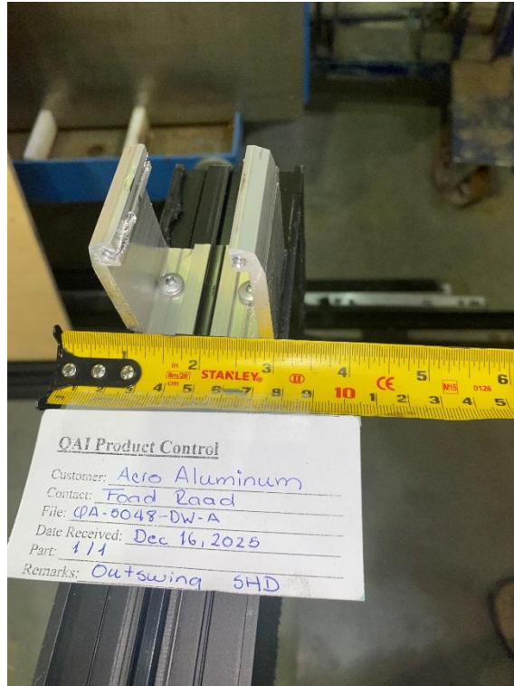
Figure 9: Door slab corner key.
