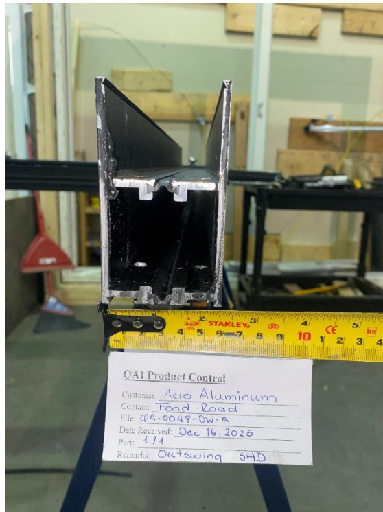
Figure 2: Top and bottom rail profile.
