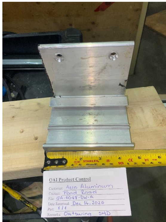
Figure 6: Frame corner key.
