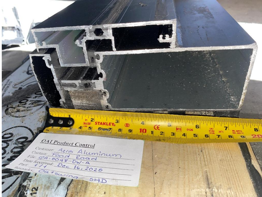
Figure 1: Frame and sub frame profiles.
